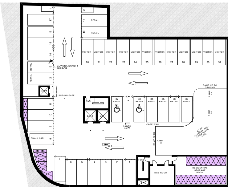
BASEMENT 01 1:400 BASEMENT STORAGE DIM: MIN 1000x1800
