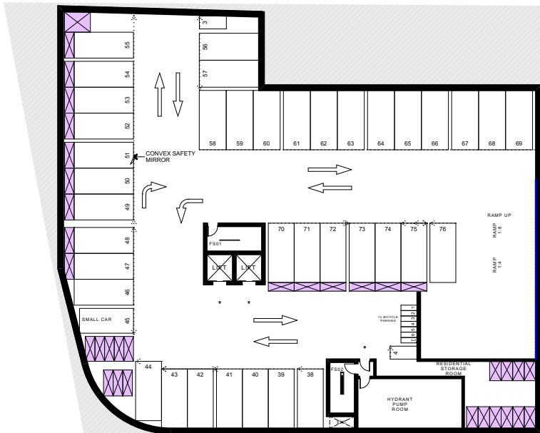
BASEMENT 02 1:400 BASEMENT STORAGE DIM: MIN 890x2400
